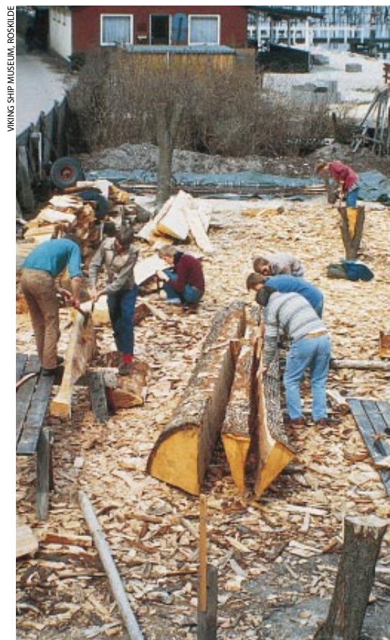
CROSS SECTION OF LONGSHIP and raw materials show ingenuity in construction. The straight tree provides angled knees, used to brace the frames. The curving tree furnishes hull-hugging frames as well as stem posts and stern posts. The oak heartwood provides the T-shaped keel. Thanks to the technique of splitting green logs in a radial pattern ( re-created by neo-Vikings, below right ), all hull planking had the same cross section, which guaranteed uniformity of strength and resilience throughout the ship.
